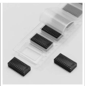
Compact single-piece board-to-board connector. The connector is to be mounted on a PC board, then another board is to be connected by being pushed against the connector.
